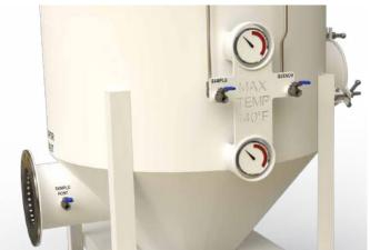
6. Locate a dependable water source with 20 GPM @ 40PSI and connect a water hose from it to the Liquid Quench Valve located on the side of the Vessel . Have the Liquid Quench Valve handle in the closed position and turn on the water source to the water hose, pressurizing the hose. This will ensure water is available to cool down the carbon in the event the carbon temperature exceeds the recommended operating temperature.
